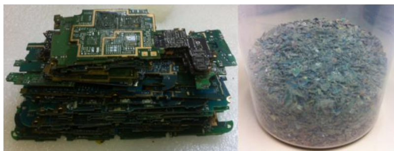
Figure 2. Printed circuit boards before and after milling
